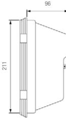
**Bipolar** U607 and P053 Dimensions in mm
